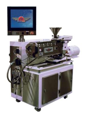
These extruders are designed to produce precision medical tubing within the space limitations that often exist in clean rooms. The unique Compact MD series extruder is designed specifically for clean room and/or controlled environments.
